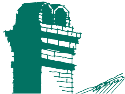
Chimney with Contrasting Courses
